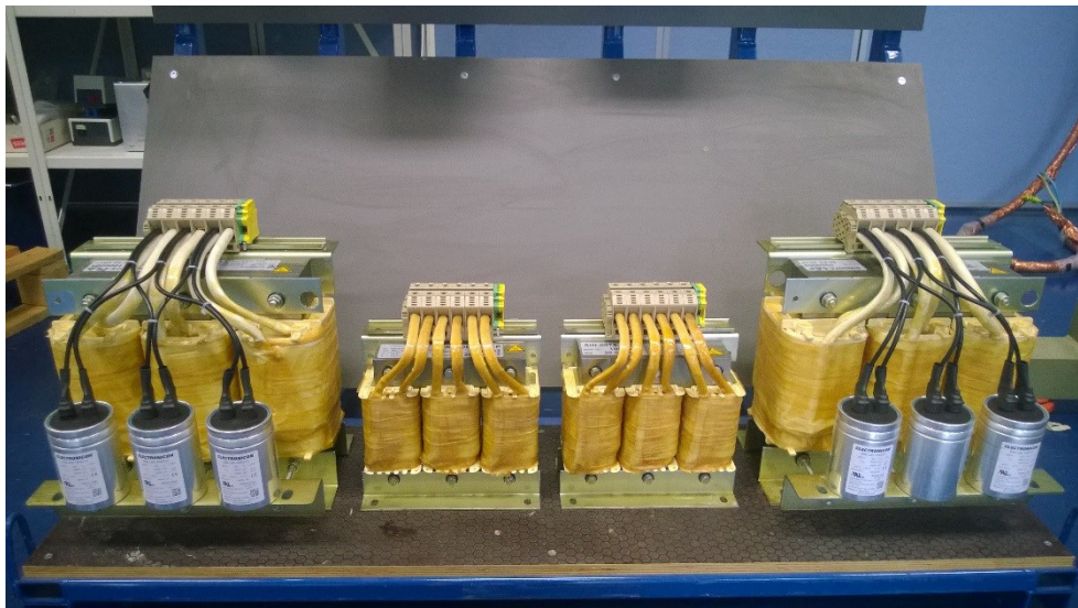
Figure 3.4. LCL filter in right is generator side and the left LCL filter is the motor side.
