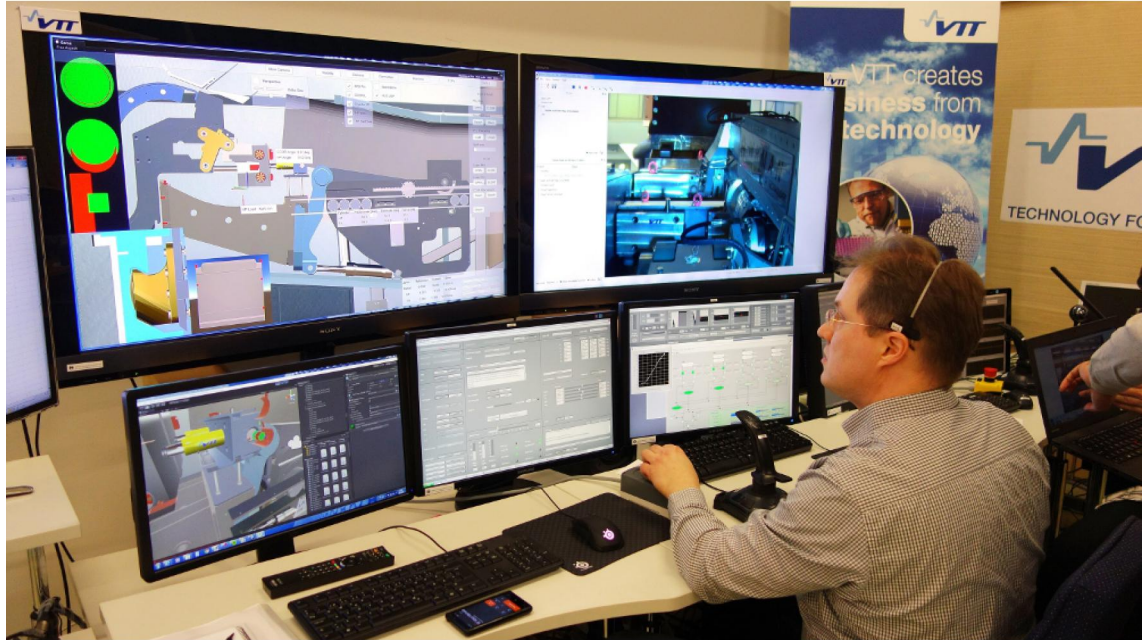
Figure 3.1 DTP2 control room at VTT. The remote handling operations are possible with the accurate simulations and virtual reality systems based on data acquired from the real equipment. [6]
