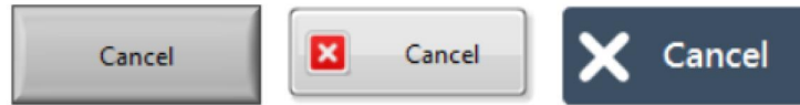
Figure 5.1 Different cancel buttons in LabVIEW. Button on the left is the classic style button, button on center is the silver style button and button on the right is the modern flat style button. The prototype version is made with classic style. The flat style button is third-party add-on provided by DMC.
