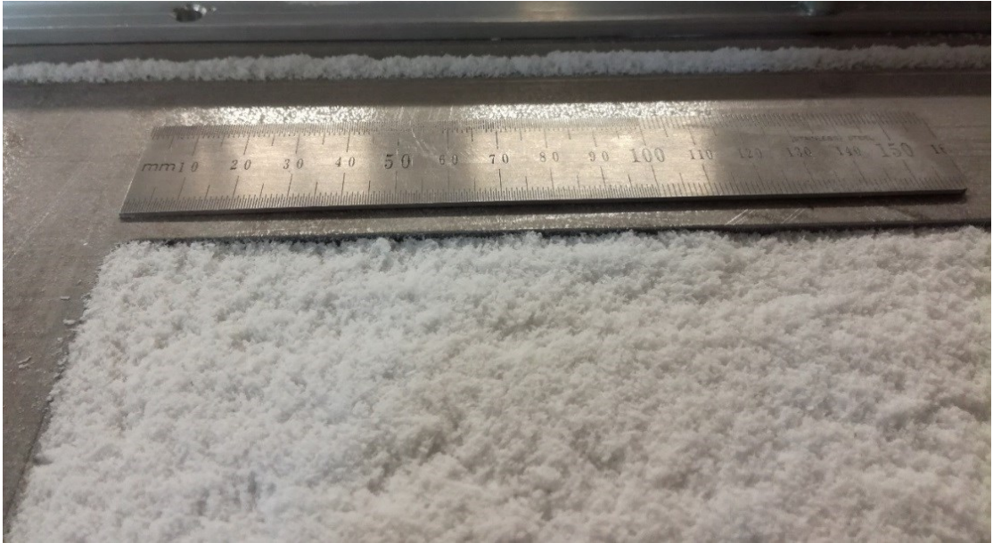
Figure 6.16. The powder bed of the PP-1 powder with 1 mm layer thickness (provided by Aalto University).
