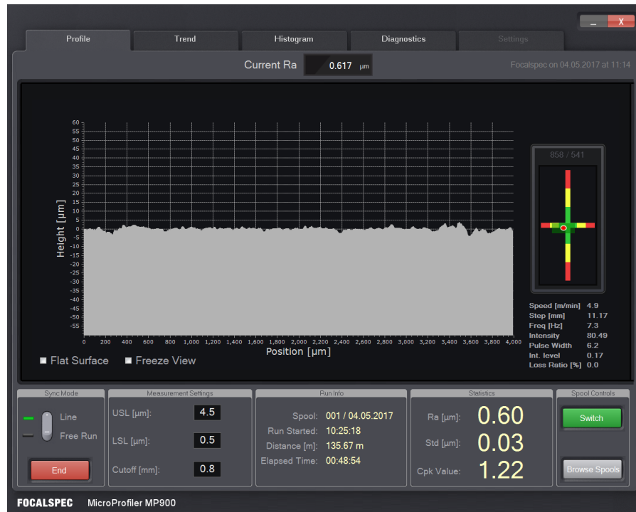
Figure 36: MP900 user interface during a line-mode measurement
