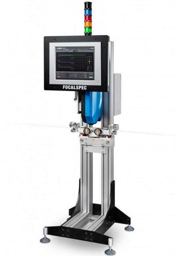
Figure 35: FocalSpec MP900 roughness measurement system [37]
