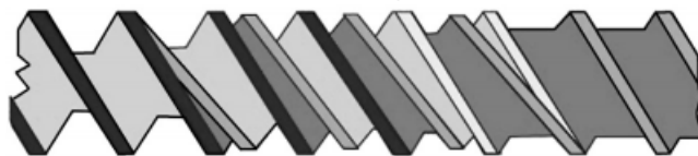
Figure 6: Barrier screw transition section, modified from [2, p. 75]
