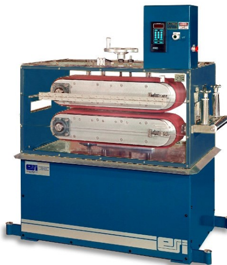
Figure 13: ESI MD series caterpillar puller [6]
