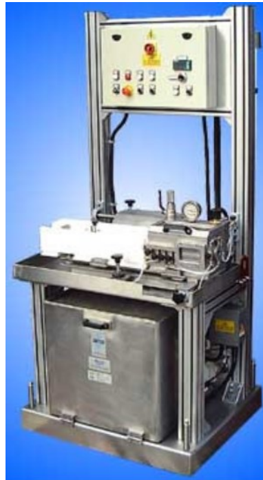
Figure 16: Gimac vacuum calibration unit [9]
