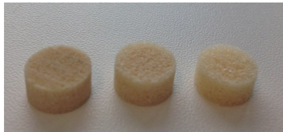
Figure 14. PU foam samples of densities 320\text{ kg/m}^3 , 160\text{ kg/m}^3 and 80\text{ kg/m}^3 .
