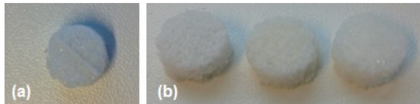
Figure 13. PET foam sample with welding line (a). PET foam without welding line having different densities ( 210 \text{ kg/m}^3 , 135 \text{ kg/m}^3 and 100 \text{ kg/m}^3 ) (b).
