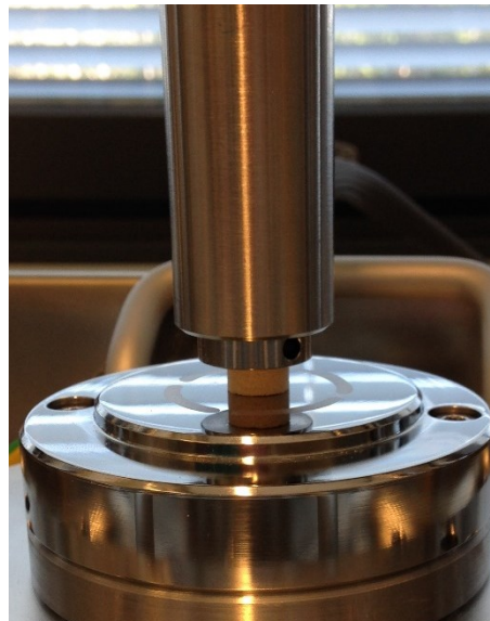
Figure 23. PU foam sample and starting position of a compression test.
