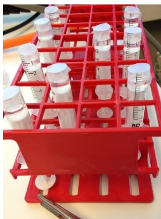
Figure 15. Hydrogel samples gelling in molds.
