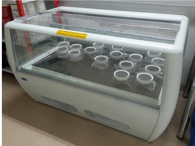
Figure 16. Test arrangements for antifog level evaluation.
