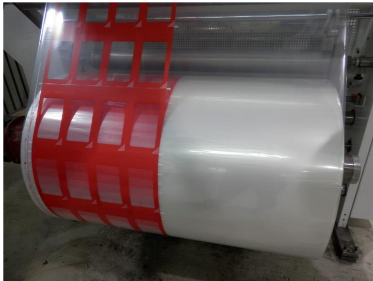
Figure 22. Surface printed AF film after AF lacquer coating process.
