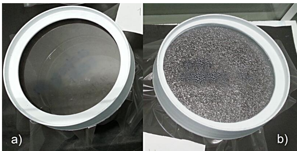
Figure 7. a) Plastic film with AF property, b) Plastic film without AF property.
