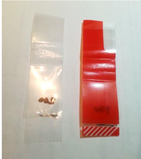
Figure 17. Sealing strips for seal strength measurements.
