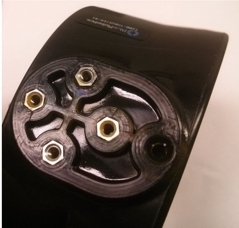
Figure 5: Cracks around thruster mounting nuts
