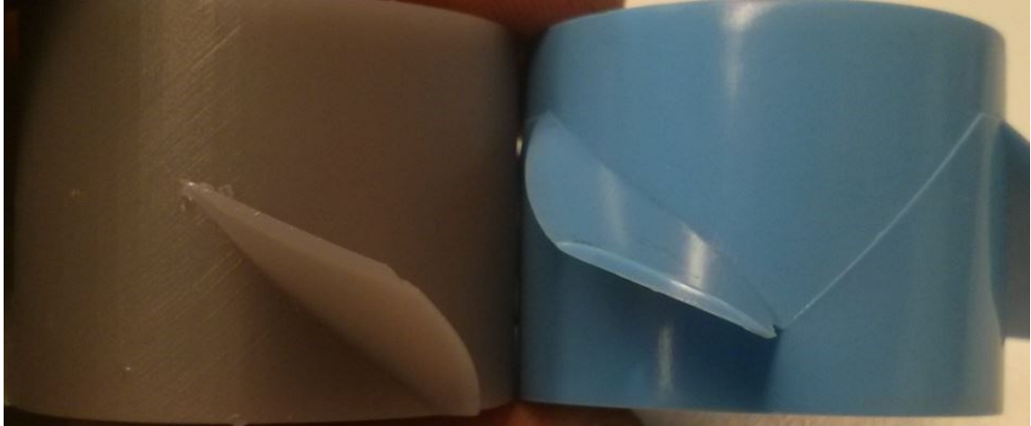
Figure 6: Reverse-flow propeller and stock one compared
