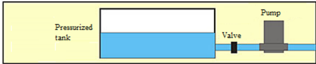
Figure 3: Pressurized tank system
