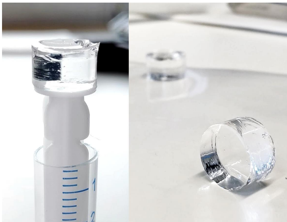
Figure 7.1. Cylindrical samples ( V = 875 \mu\text{l} ) for the unconfined compression testing were prepared in cut 5 ml syringes.
