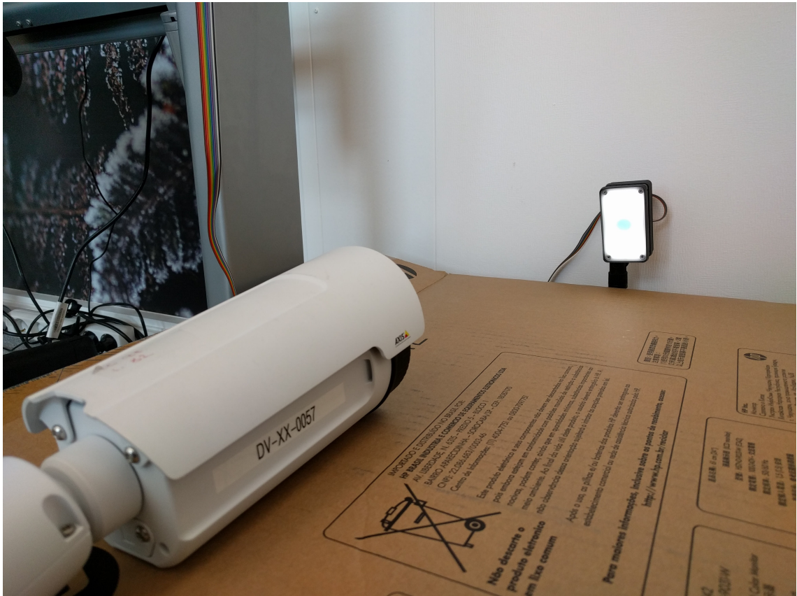
Figure 4.2 Latency measurement setup of the camera and LED target using the OptoFidelity Video Multimeter.
