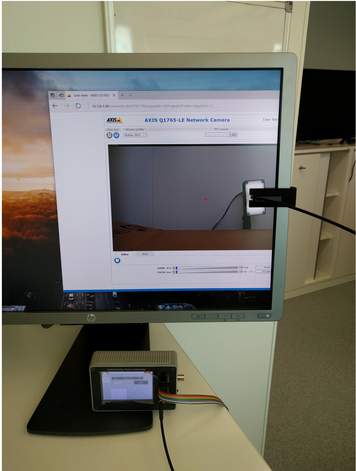
Figure 4.1 Latency measurement setup of the display using the OptoFidelity Video Multimeter.
