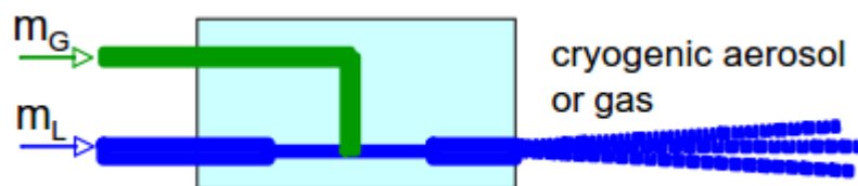
Figure 21: LIN-GAN cryofluidic nozzle. m_G = gas stream, m_L = liquid nitrogen stream [84].
