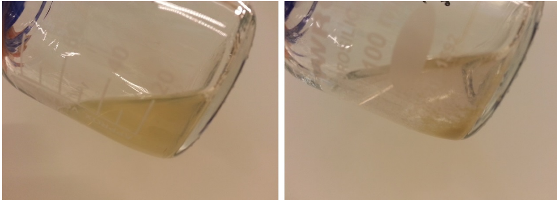
Figure 6.11 Photos of two sample bottles after the sulfide oxidation experiment 3 with setup B. Left photo shows a sample with only effluent, right photo shows a sample with effluent and inoculum.
