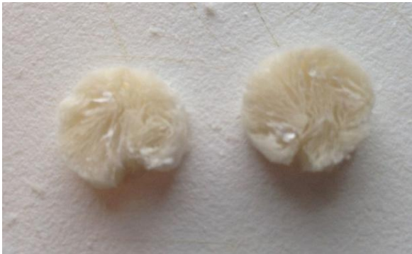
Figure 4.2 Porous scaffolds of chitosan-BAG 75wt% composite samples.
