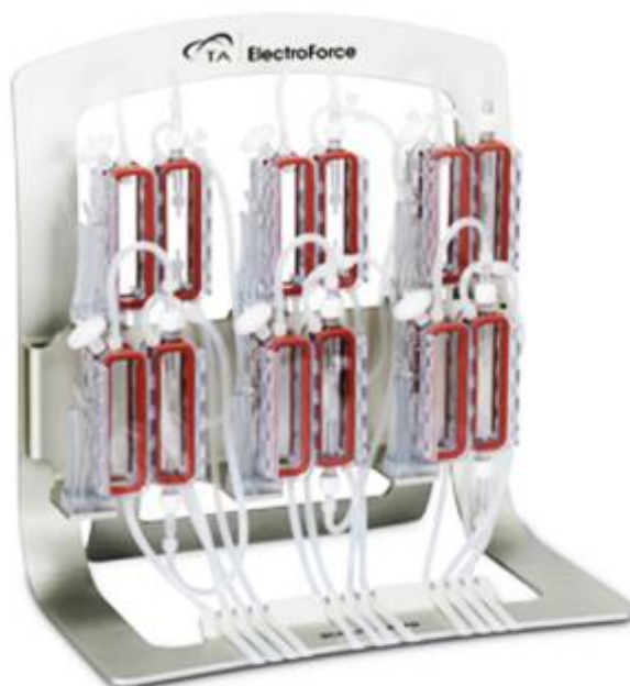
Figure 10. TA Instruments 3D CulturePro Bioreactor system for multiple single samples [169].
