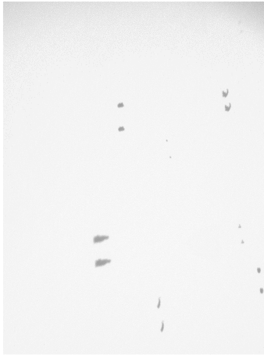
Figure 6.4. Double exposed picture of particles falling in the reactor.
