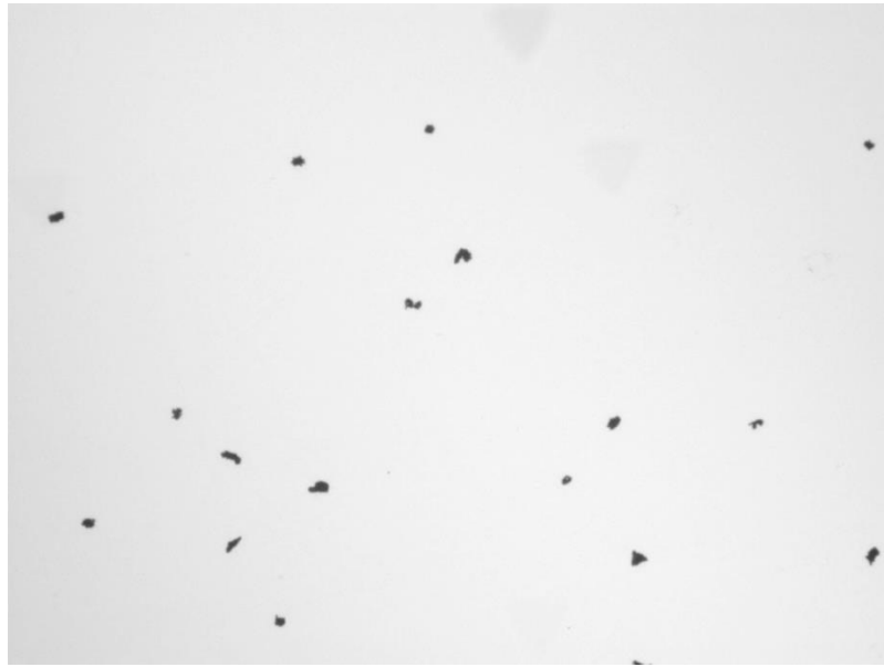
Figure 7.27. Particles of B1a after pyrolysis experiment in 900 °C, drop-height 17.5 cm.
