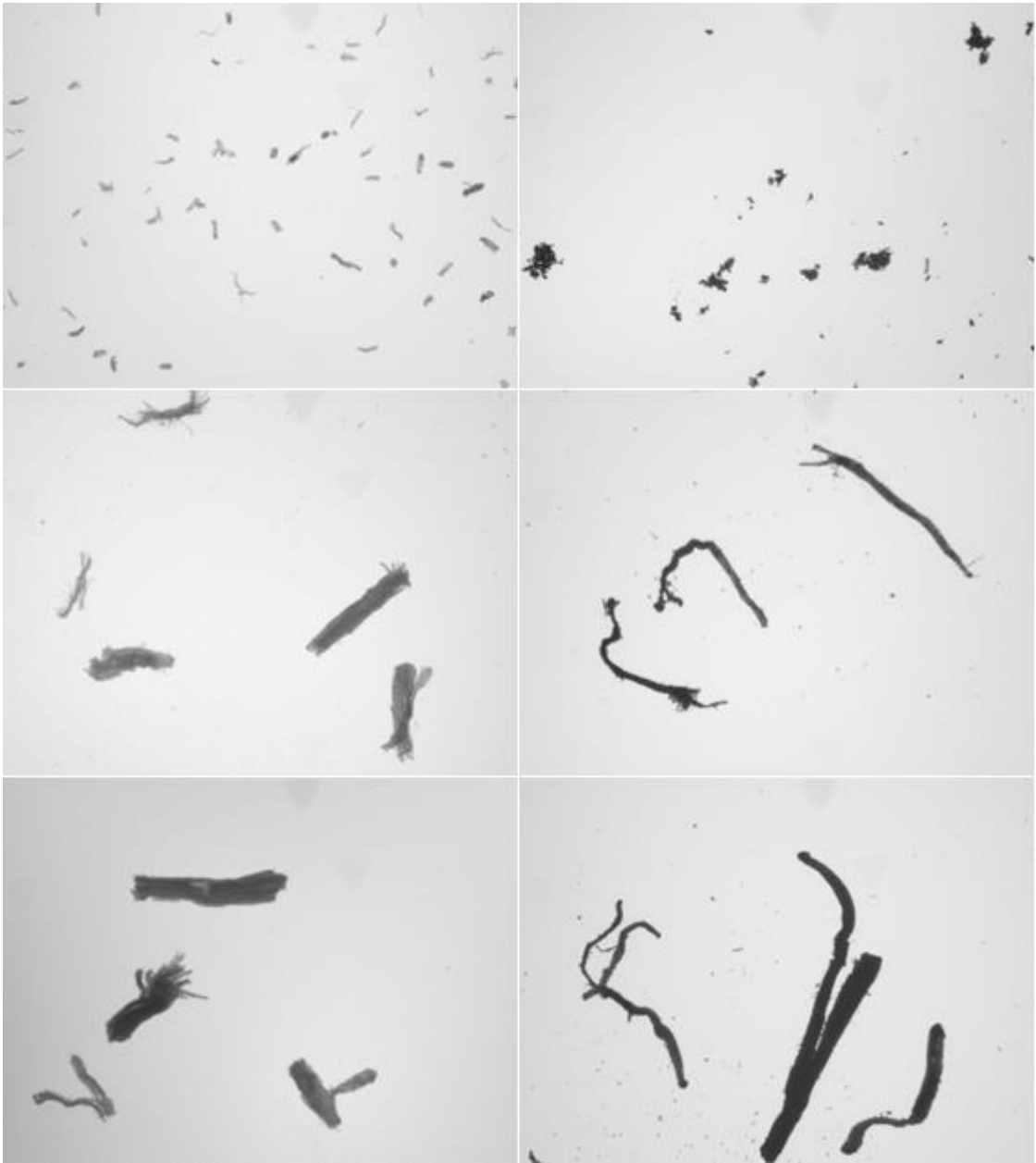
Figure 7.11. Pictures of particle projections on the light diffuser plate: On the left biomass B1a, B1b and B1c, and on the right B2a, B2b and B2c, respectively.
