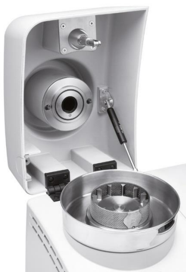
Figure 6.1. The Retsch mill ZM 200 used by TUT [69].
