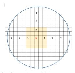
Figure 8.7 Well map of imaging coordinates. Each square represents the area of well that is seen in live mode with 10x magnification on the operating panel of BioStation CT.
