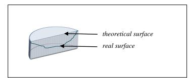
Figure 8.10 Schematic illustration of the shape of a hydrogel sample, cut into half. Hydrogels could be theoretically imagined to form a cylinder shaped sample with flat surface when gelated into a well plate. In reality, the surface of the hydrogels curved down from the edges to the middle of the sample: difference in the thickness was up to several hundred micrometers. In addition, the surface topography was uneven in smaller (micrometer) scale.
