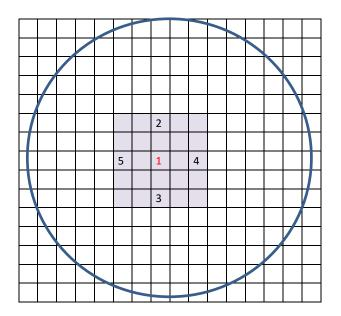
Figure 8.9 Recommended map of imaging points in a well. The colored area corresponds to the area where cells were mostly located. In imaged points outside this area, cells were usually not present, hence images should be acquired from coordinates 1-5, or other points with similar distance from the center of the well (point 1).
