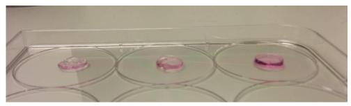
Figure 8.5 Gellan gum hydrogels transferred from 5 ml syringes to well plate lid for imaging with ApoTome. On the left 145  $\mu$ l, in the middle 200  $\mu$ l and on the right 290  $\mu$ l samples.
