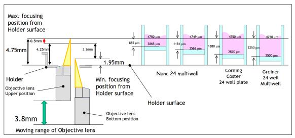
Figure 8.8 Focusing range in BioStation CT, and effective focusing ranges when using well plates from different manufacturers. (Picture: Yasujiro Kiyota, Nikon, reproduced with permission.)
