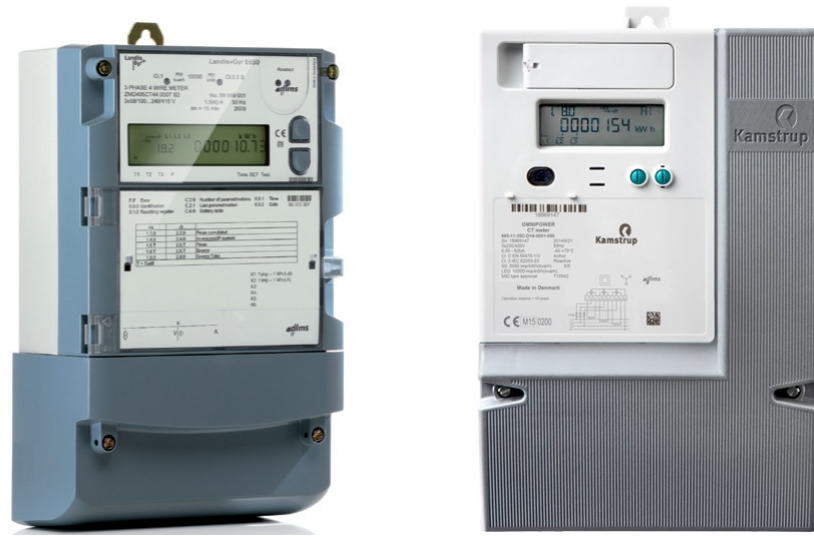
Figure 4.11 Smart meters included in the demonstrations. On the right side Landis+Gyr E650 [28] and on the left side Kamstrup Omnipower [29].
