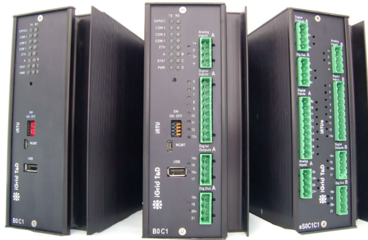
Figure 4.10 Different device models from the iRTU series: iGW-B0C1 unit (left), iRTU-B0C1 unit (middle) and iRTUe-S0C1C1 unit (right). [27]
