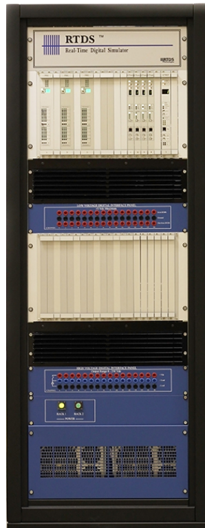
Figure 5.2 Real-Time Digital Simulator cubicle[57]
