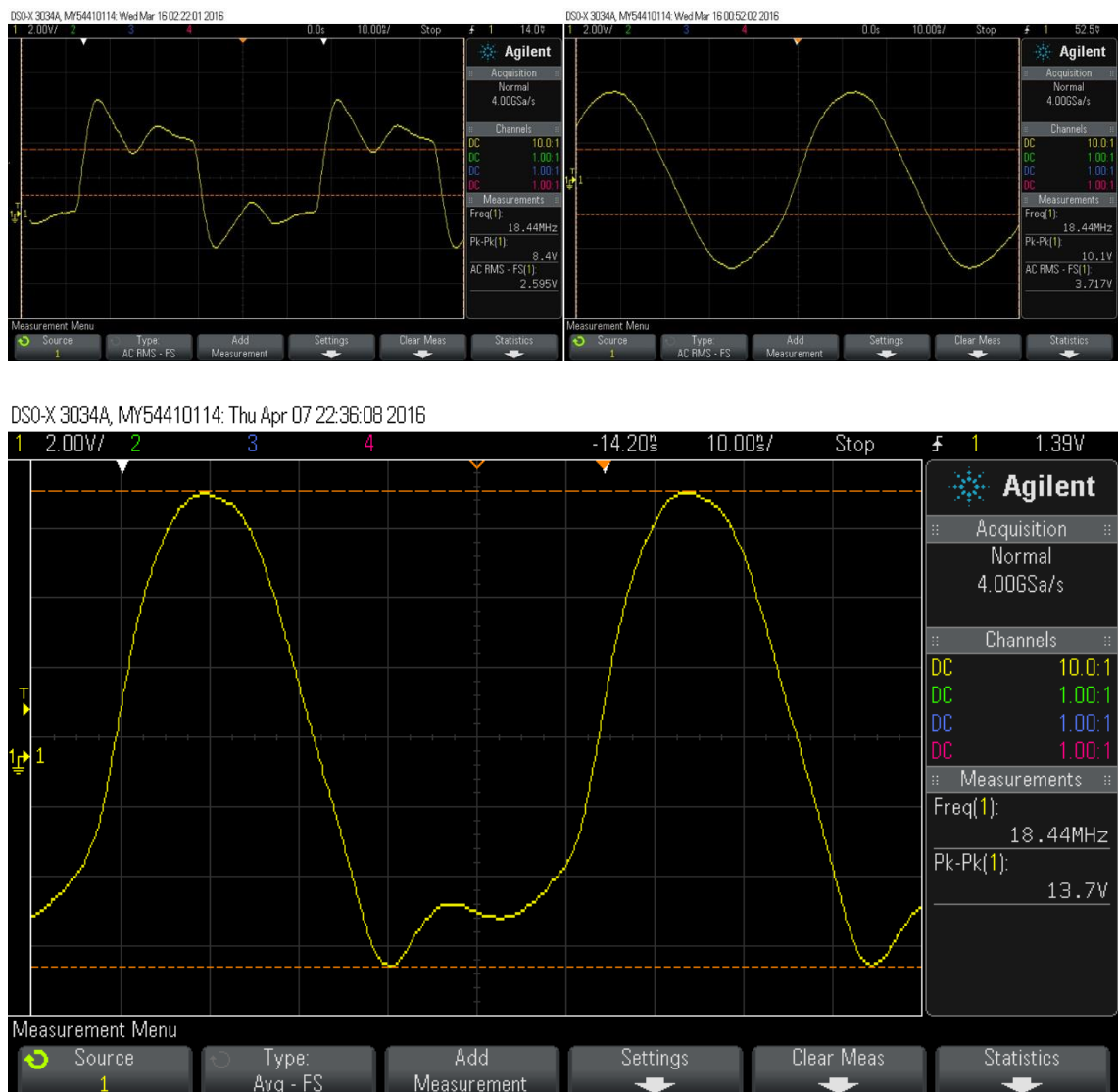
Figure 47 Oscillator output waveforms comparison.
