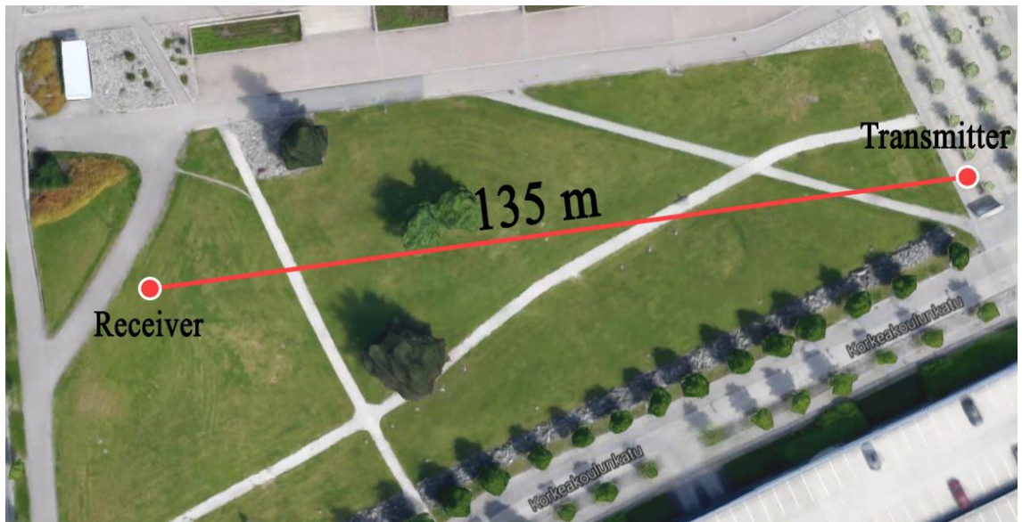
Figure 54 Approximate distance (135 m) reached by the PCB transmitter.
