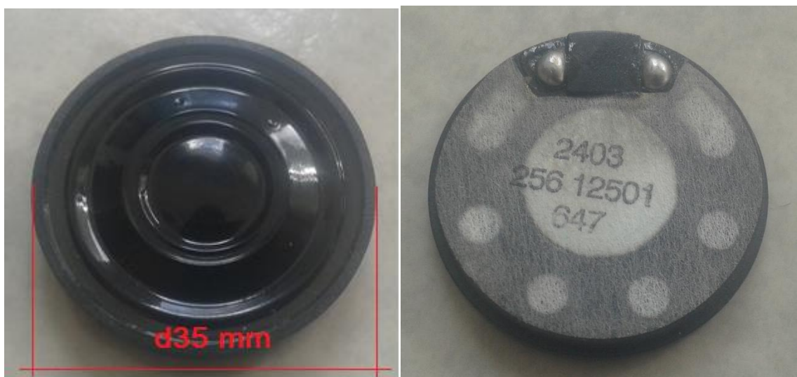
Figure 11 Speaker top (left) and bottom (right) views.
