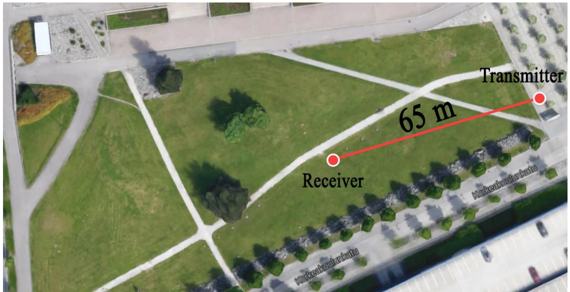
Figure 53 Approximate distance (65 m) reached by the original transmitter.
