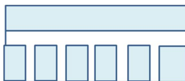
Figure 3.5. A patterned ITO plate. White regions are of glass and the blue ones of ITO.
