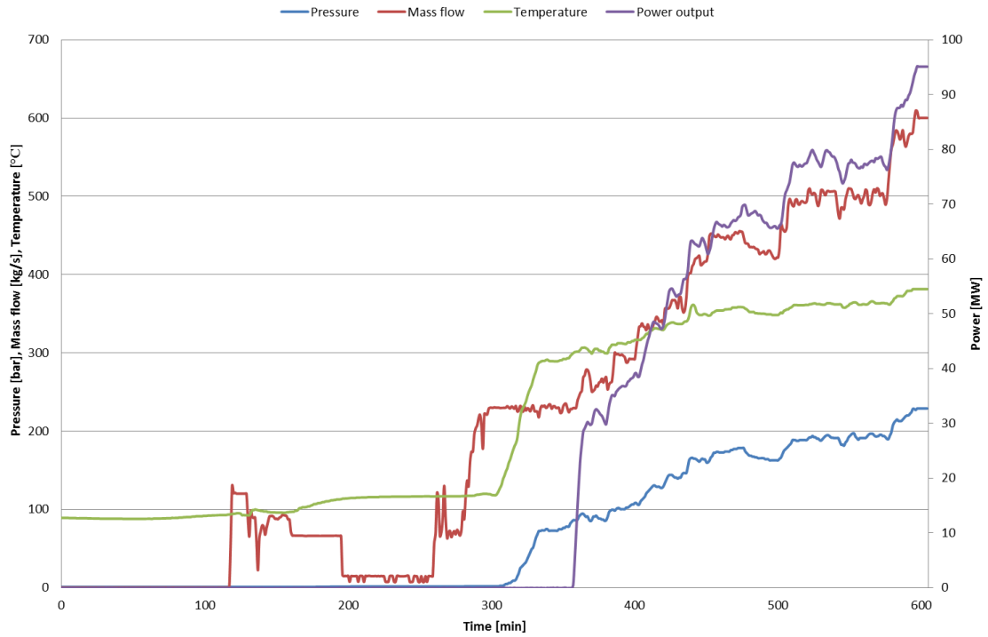
Figure 33. Measured variables in water separator during the cold start.
