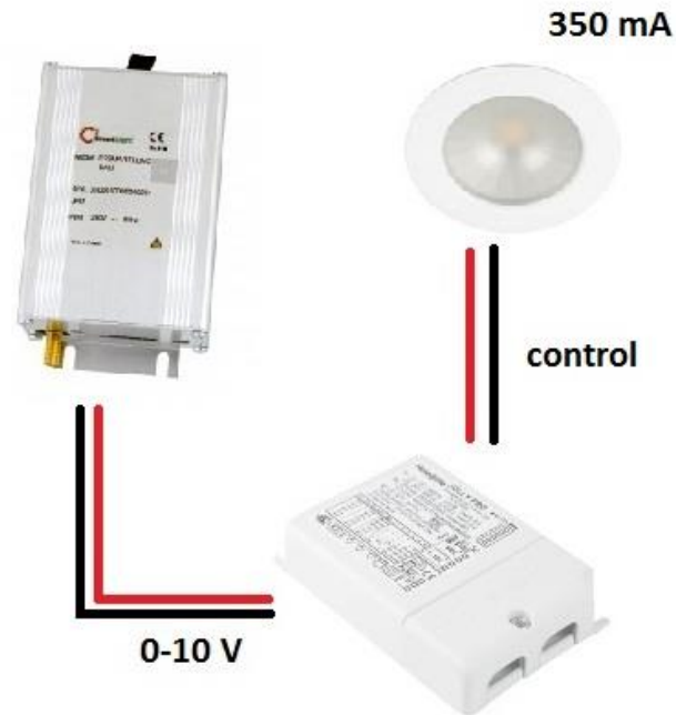
Figure 11. Hardware setup of Light Management Tool.
