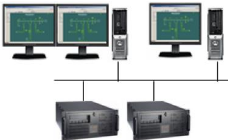
Figure 2-8 A simple system with two system servers located in the control center (ABB 2013).
