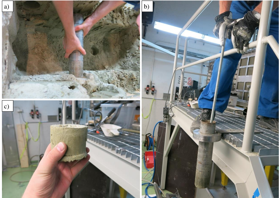
Figure 40. Pellet samples close to the blocks were taken by using an iron pipe (a), and custom-built instruments (b) were used to take the samples (c) out from the pipe.
