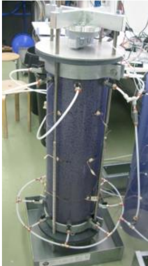
Figure 23. Test cylinder comprised of a PVC cylinder fitted with plastic pistons at the bottom and top. The diameter of the test cell was 269 mm and the height was 800 mm. Flow inlet and outlet ports (inner diameter 6 mm) were found at the bottom and top of the test cylinder, respectively. (Pintado et al. 2013)
