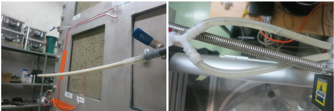
Figure 53. Burst of bentonite caused blockages in the outflow pipes.
