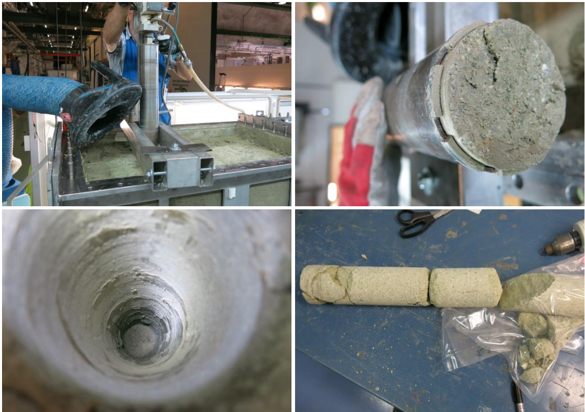
Figure 39. Backfill block drilling.
