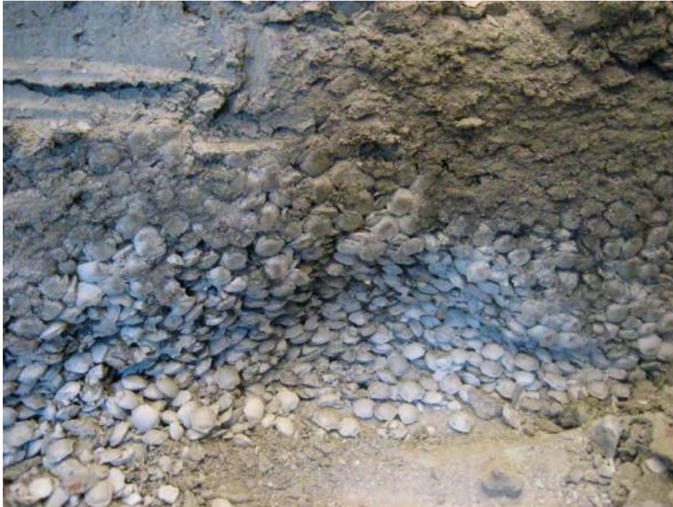
Figure 21. Dry and wet MX-80 pellets in a test performed to study effects of water inflow on the buffer (Åberg 2009).
