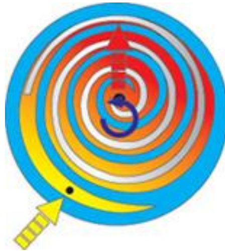
Figure 4.9: Scroll Pump Operation [28]
