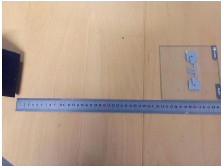
Figure 8.2: Tag placed 40 cm from the Reader Antenna
