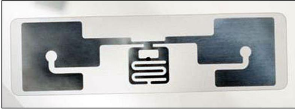
Figure 4.4: Dogbone tag made with RFMicron's Magnus S Sensor [29]
