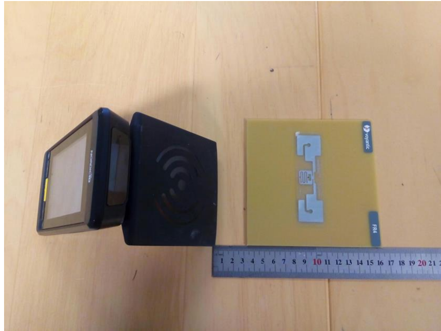
Figure 5.2: Tag placed 10 cm apart from reader antenna
