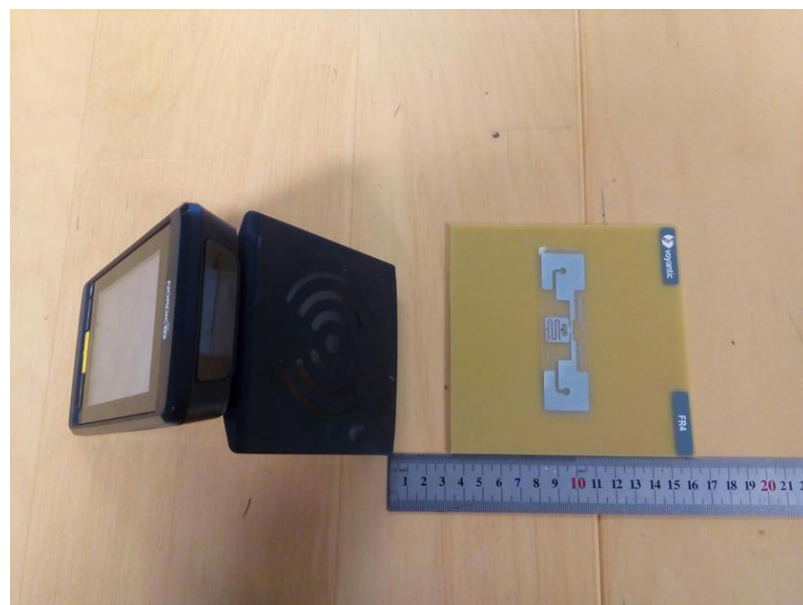
Figure 8.1: Tag placed 10 cm from the Reader Antenna
