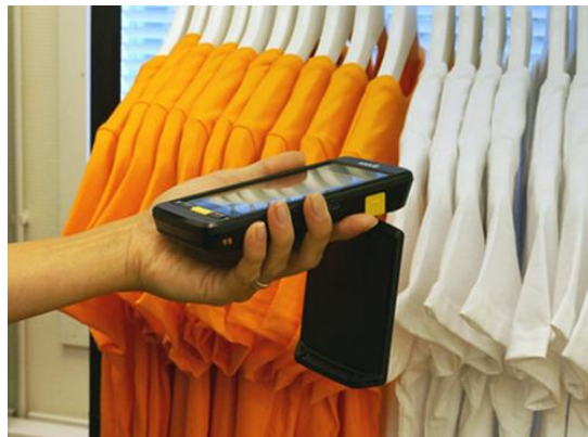
Figure 4.6: Nordic ID mobile reader used to read RFID tags in a textile factory [29]
