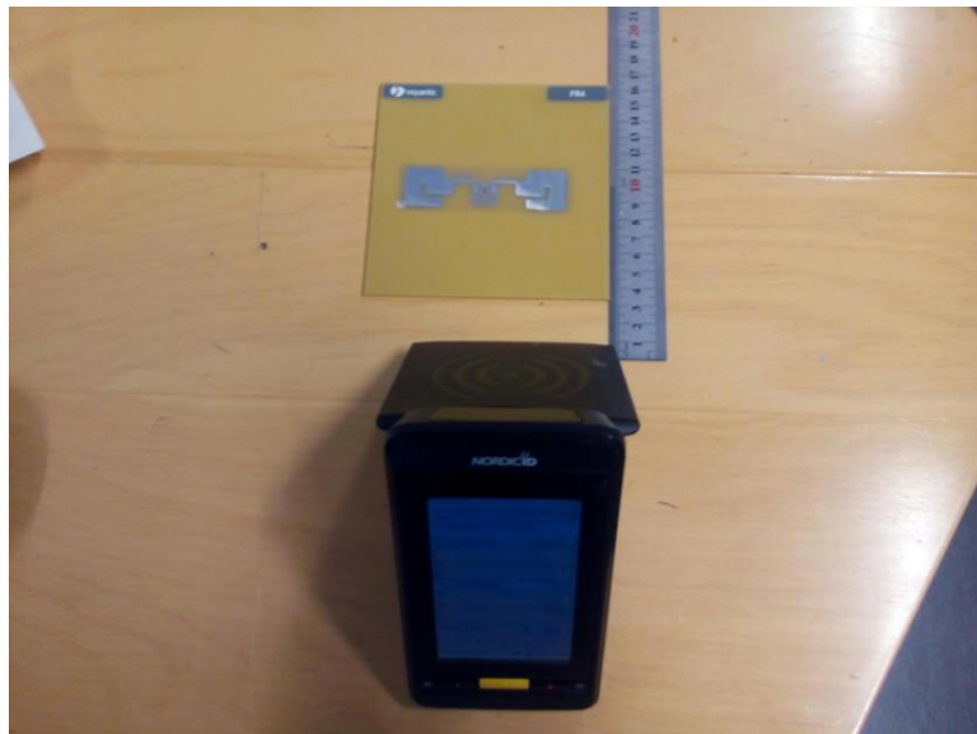
Figure 5.3: Readings taken when a dab of Acetic acid is placed on the tag that is 10 cm away from the Reader Antenna
