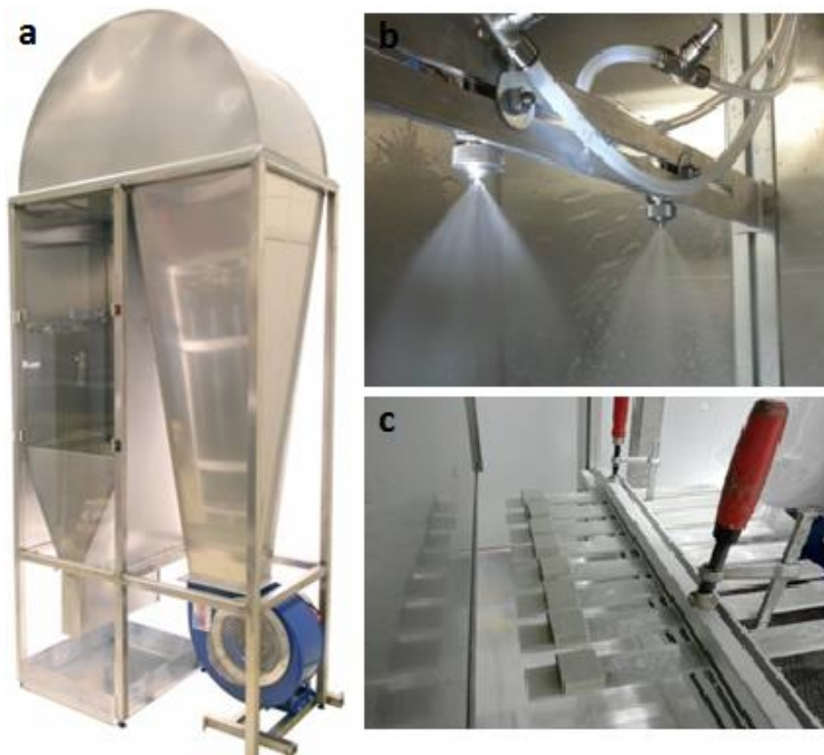
Figure 50. a) Icing wind tunnel, b) nozzle system inside the wind tunnel and c) typical set of samples with masks at TUT.
