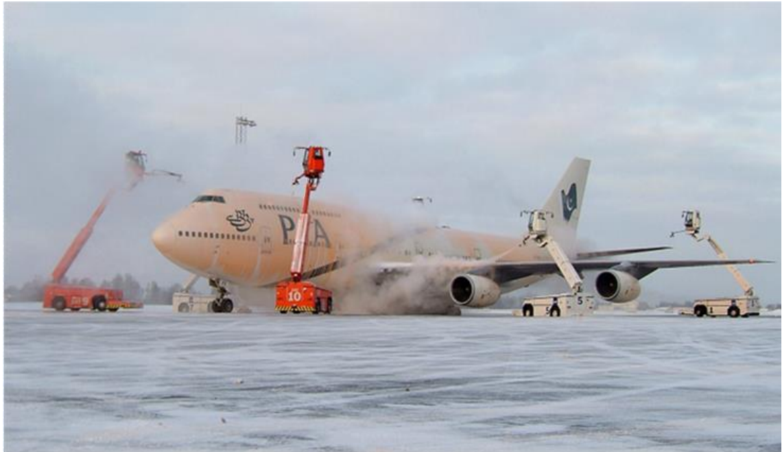
Figure 4. De-icing of the airplane with de-icing chemicals. [21]
