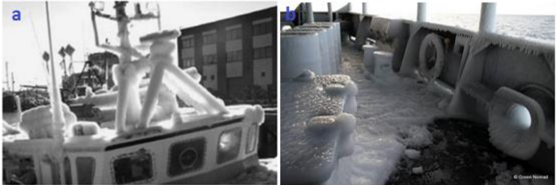
Figure 5. Effect of severe icing on sea vessels' structures. a) Superstructure icing is covering the radar and communication antennas of the small ship [12] and b) heavy icing of the deck. [25]
