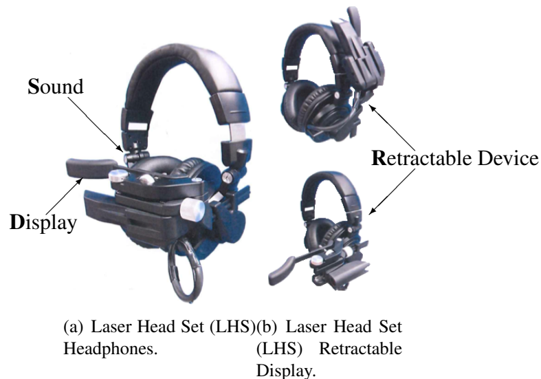
Figure 2.13: Images taken from pamphlet given in Mobile World Congress 2013. (a) Laser Head Set (LHS) giving a perspective of the device [QDL13]. (b) Small screen adjustable in device Laser Head Set (LHS) [QDL13].
