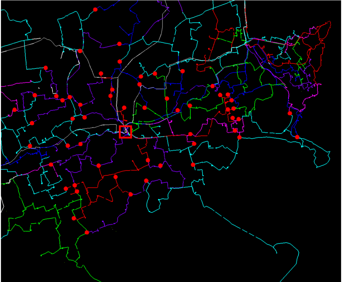
Figure 7.3. Case 5 for urban area. Remote controlled disconnectors are highlighted with red dots and primary substation with red square.
