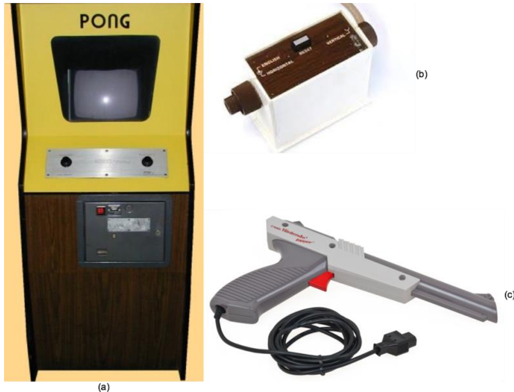
Figure 1.1 Some of the early methods of input in video games. (a) A pong arcade machine, utilizing 2 rotating dials (source: pong-story.com), (b): the two-knobs controller for the Magnavox Odyssey console (source: ign.com), and (c) the Nintendo Zapper Gun (source: Wikipedia)
