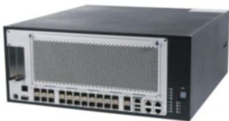
Figure 4. BCN module used to build Multicontroller BSC configurations [28].
