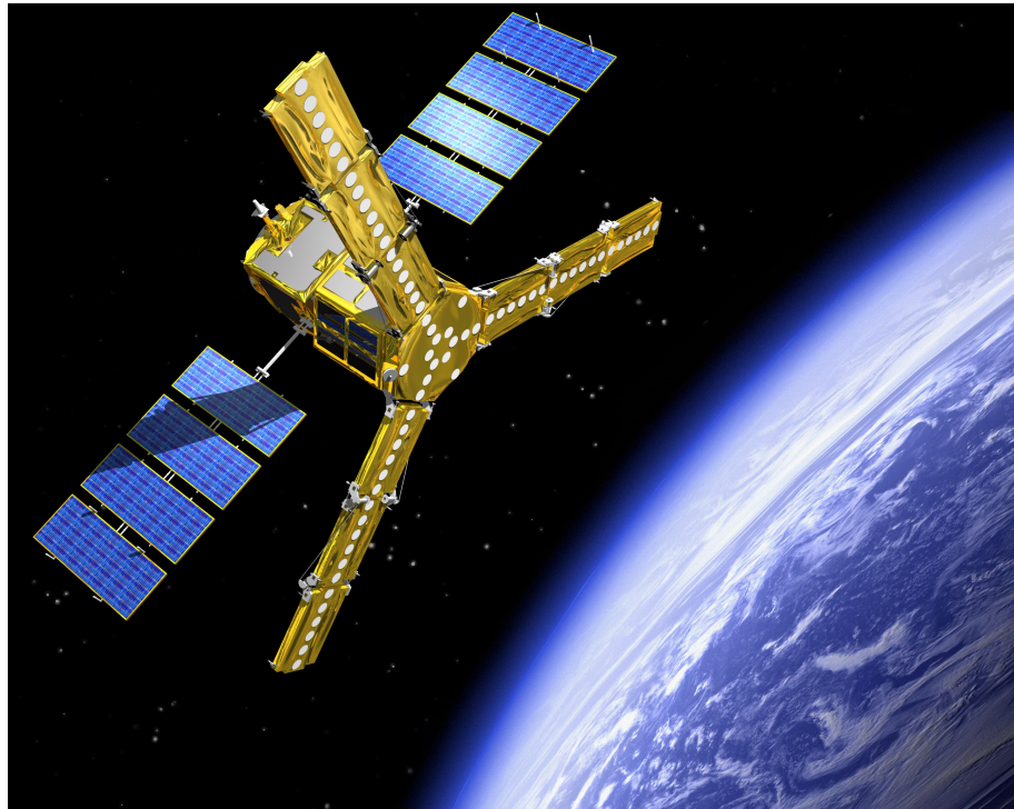
Figure 2.5 An artistic view of the SMOS satellite, showing the Y-shaped form of the instrument [45].
