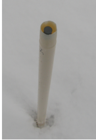
Figure 2.1 A frost tube with the inner tube inside the outer guide without the protective cap.
