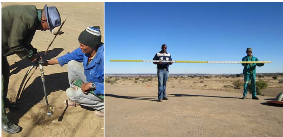
Figure 3.2. Water pressure measurements and water level measurement tool (Tuovinen)
