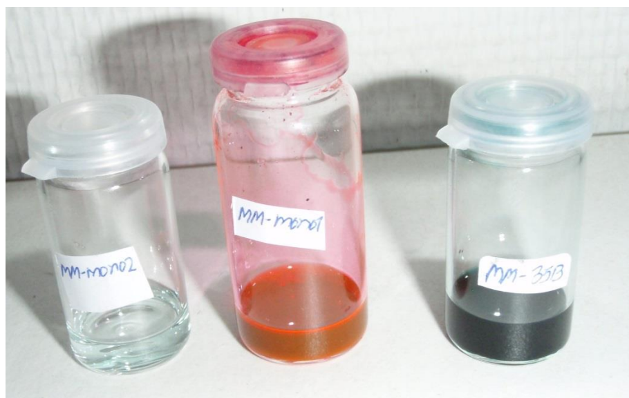
Figure 12. Colors of the dibromotetrafluoro monomer (left), DPP monomer and polymer product (right). All solutions are in tetrahydrofuran.
