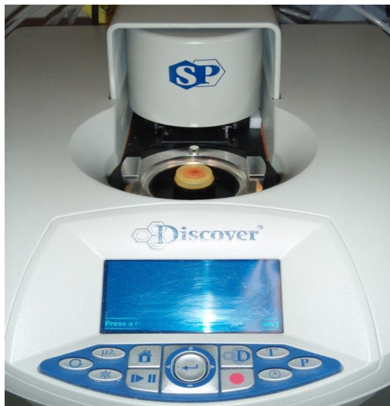
Figure 10. Monomodal microwave oven used in laboratories. Reaction chamber is in the middle of the picture and control panel in front.
