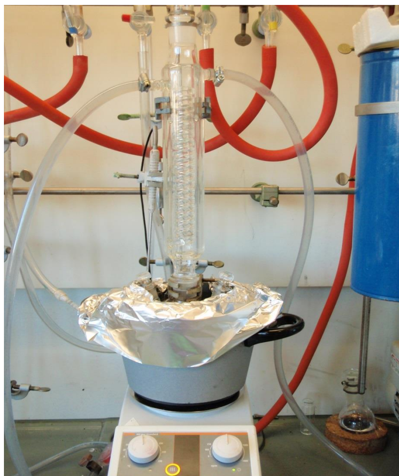
Figure 11. Reaction arrangement for the monomer synthesis.
