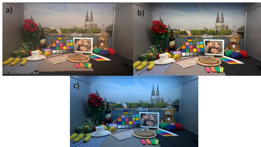
Figure 2.9: Unbalanced images from same scene: a) halogen lightning, b) florescent lightning, and c) daylight lightning.
