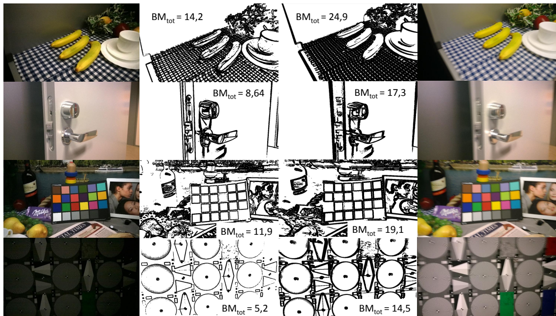
Figure 5.4: Comparison between no-blur and blur images, where BM_{tot} values are calculated with the method described in Figure 5.3. Edge-images are presented as negative images in order to achieve more pleasant look.
