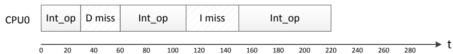
Figure 5.6: Example of a cache definition for processing element. Distributions used in the definition randomly chooses the amount of clock cycles to the next cache miss. That amount is generated again every time cache miss occurs. Timeline shows a task executing 160 integer operations on a PE cpu0 . The execution is stalled for 30 cycles due to data cache miss and 40 cycles for instruction cache miss, and thus taking 230 cycles to complete.
