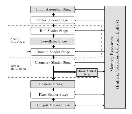
Figure 4.1: The Direct3D 11 pipeline and new features added to the API in recent versions [31, p. 4].
