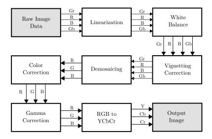
Figure 2.9: Algorithms in a typical image processing line [11].
