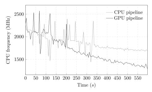
Figure 6.3: The average frequency or all CPU cores during processing.
