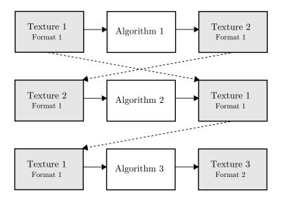
Figure 4.7: The ping-pong buffering scheme in GPU-based image processing.
