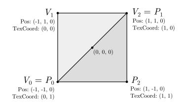
Figure 3.5: A scene description used for GPU-based image processing tasks. The first triangle is defined by vertices  $V_1$ ,  $V_2$  and  $V_3$  and the second triangle by vertices  $P_1$ ,  $P_2$  and  $P_3$ .
