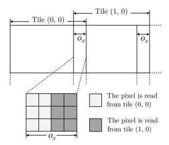
Figure 4.6: Processing output pixels when a 5x5 kernel is used.
