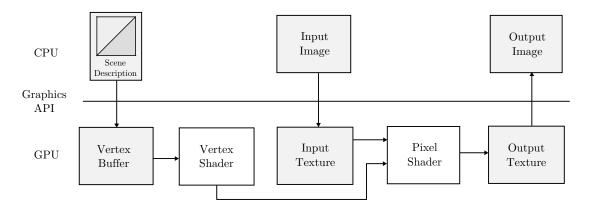
Figure 3.4: A typical processing flow in GPU-based image processing.
