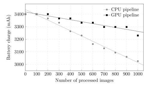
Figure 6.4: The battery charge of the test device when 1000 images were processed consequently.
