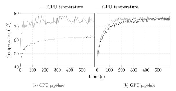
Figure 6.1: Measured GPU and CPU temperatures for (a) CPU implementation and (b) GPU implementation during processing.
