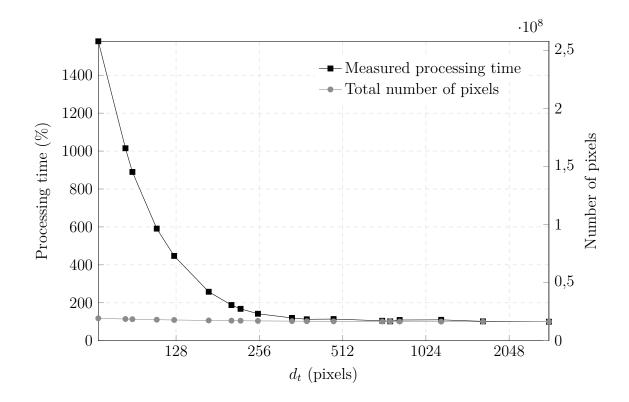
Figure 5.2: The processing time of the pipeline with different texture sizes.
