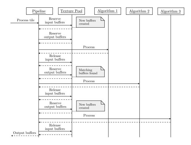
Figure 4.8: The processing flow inside the pipeline component.
