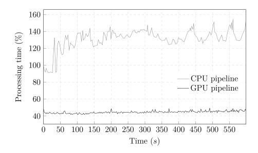
Figure 6.2: The processing time of a single image during measurements.
