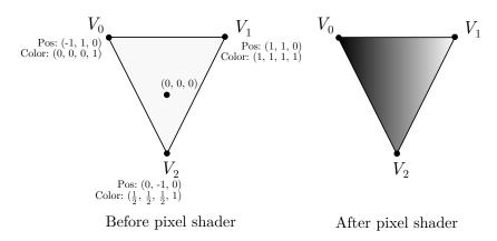
Figure 3.3: The output of a pixel shader that sets the color of the pixel directly to the color passed from the vertex shader.
