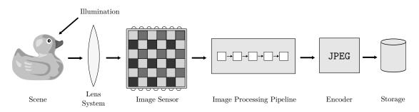
Figure 2.1: The components of a digital still camera.
