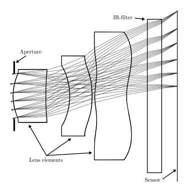
Figure 2.2: A typical mobile camera lens system [2].
