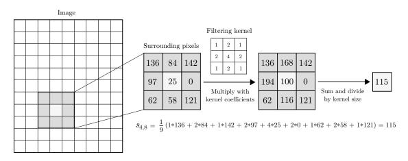
Figure 2.7: A simple blur effect using a 3x3 filtering kernel.
