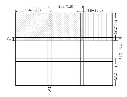
Figure 4.5: An example of dividing an image into three tiles horizontally and vertically.
