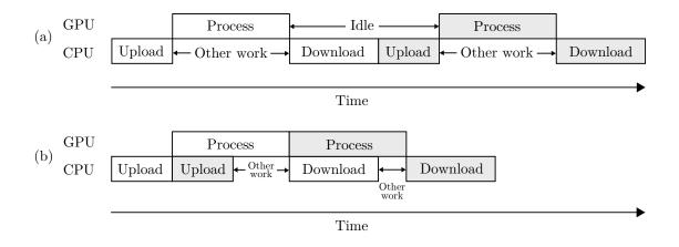
Figure 5.3: Execution timelines in cases (a) when there is no concurrency between texture transfers and processing and (b) when processing is done in parallel with texture transfers.
