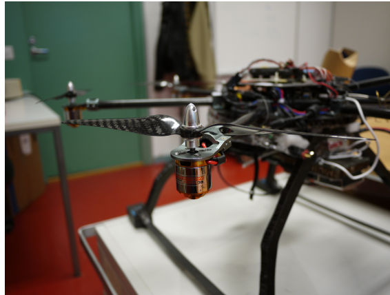
Figure 3.7: Illustrating the reversed motor mount which moves the motor and propeller to the opposing sides of the mounting plate, decreasing the moment of the force caused by imbalance propellers.
