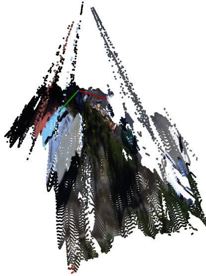
Figure 4.3: This is the point cloud extracted from disparity image presented in Figure 4.1. This image is an example of camera movement between images, resulting in incorrect calibration. Axes are scaled to 1m
