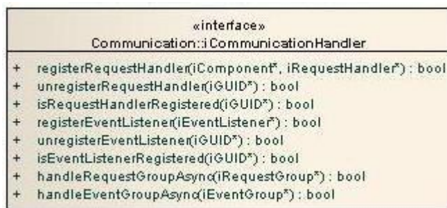
Figure 4.8. Interface that the Communication handler component reveals
