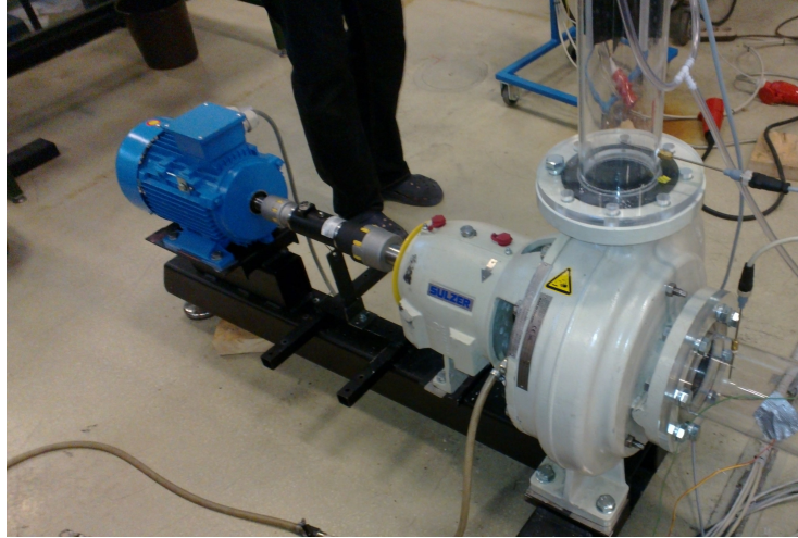
Figure 4.8: Torque transducer with assembled coupling.
