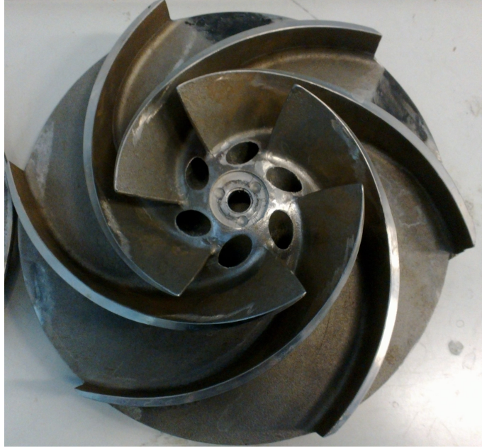
Figure 1.4: Picture of a standard semi-open type impeller of measured device.
