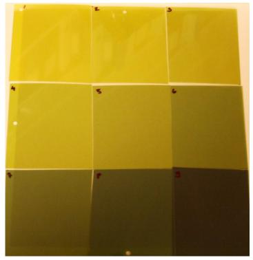
Figure 13. Irradiated films with the known doses in the same arrangement they were scanned.
