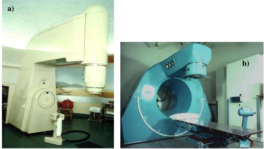
*Figure 1. a*) 4 MeV linac of 1950s from Mac-Vic, b) 6 MV linac, mid-1960s from Mullard Equipment (MEL). Adopted from [8].
