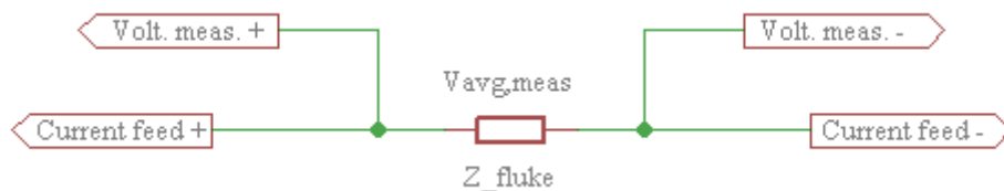
Figure 4.13 The setup of the system test with purely resistive load.
