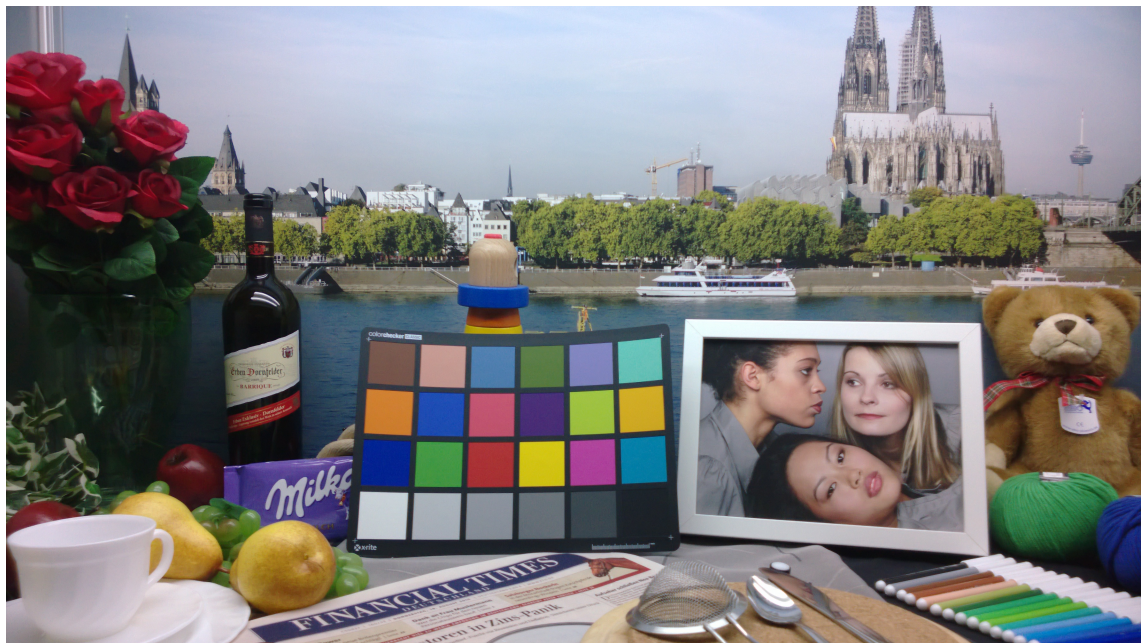
Figure 5.2: The scene used in the studio setup. The gray patch used for accuracy measurement is the second from the low left in the ColorChecker.
