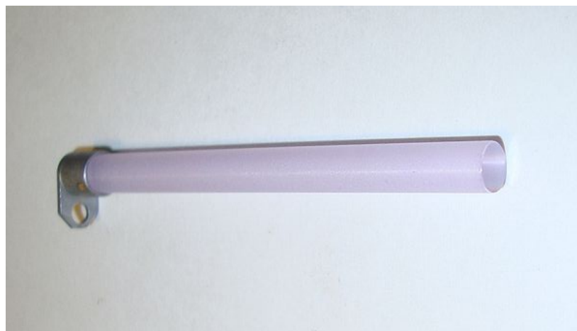
Figure 3.3: Example of Nd-YAG rod. This photo is taken from website http://en.wikipedia.org/wiki/User:Zaereth .
