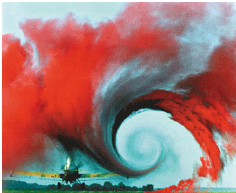
Figure 4.1: Picture showing turbulent vortex created by airplane's wing. Picture was taken from website http://www.einstein.com/tag/Aerodynamics/ .
