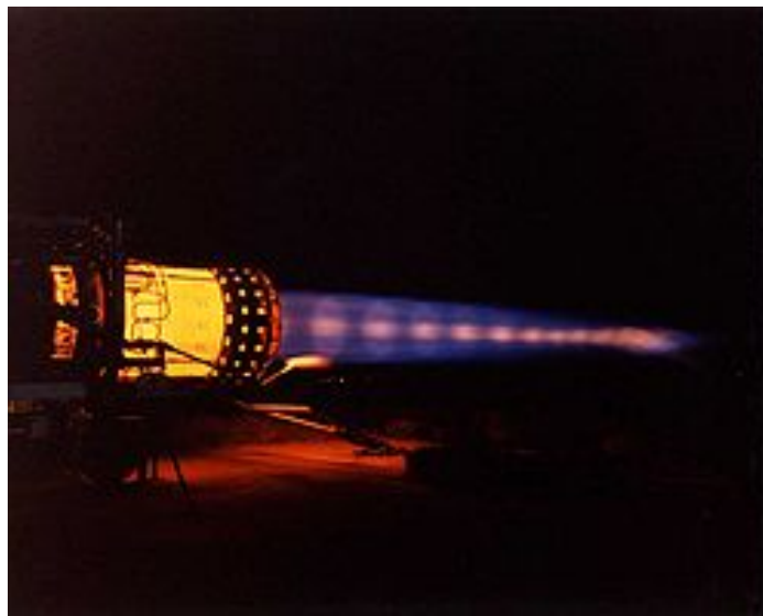
Figure 4.2: Picture showing Mach shock discs in jet stream of afterburning turbojet engine. Picture is taken from website http://en.wikipedia.org/wiki/Shock_diamond .
