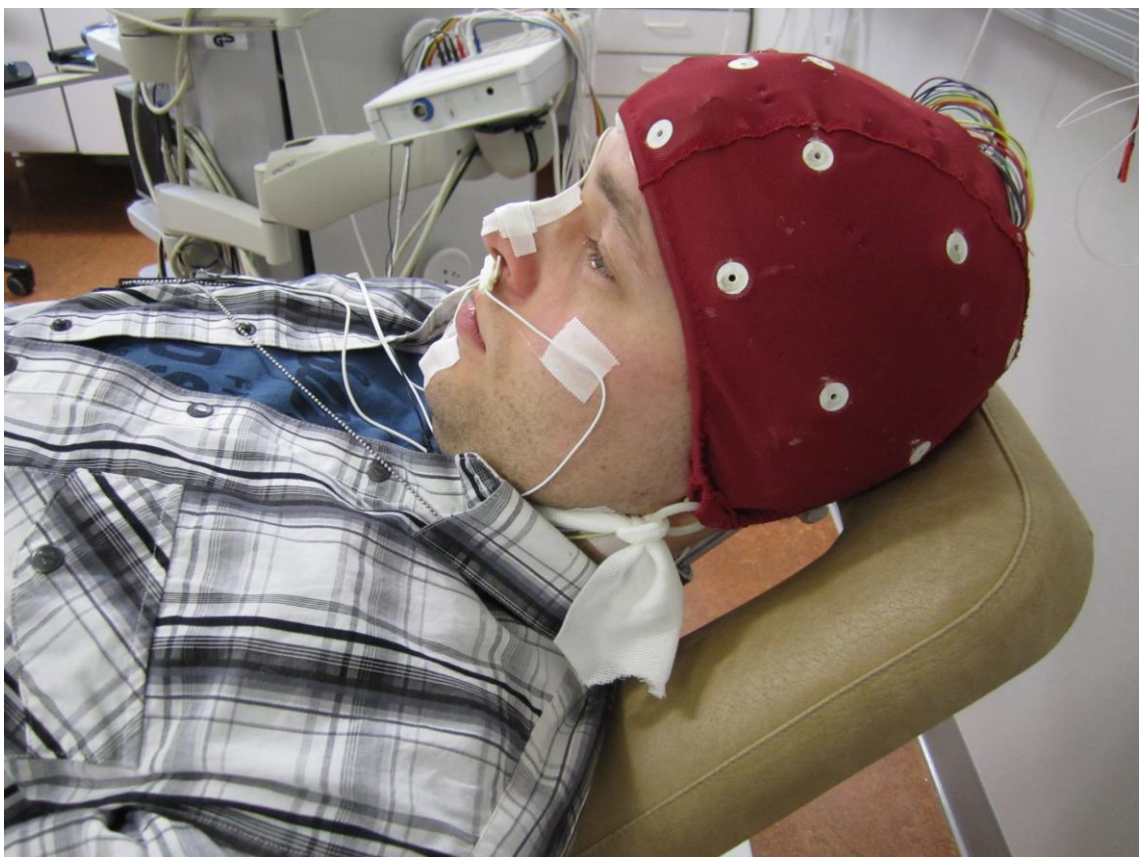
Figure 3.2. Image of the measurement setup. Separately movable part of the bed is seen under the head of the test subject. In the image the head of the test subject is lifted forward, while the body remains straight. Image is taken during the test measurements for the thesis, test subject being the author. Respiration sensor below the nose is left out from the final measurements. Amplifier used in the measurements is seen in the image next to test subject.
