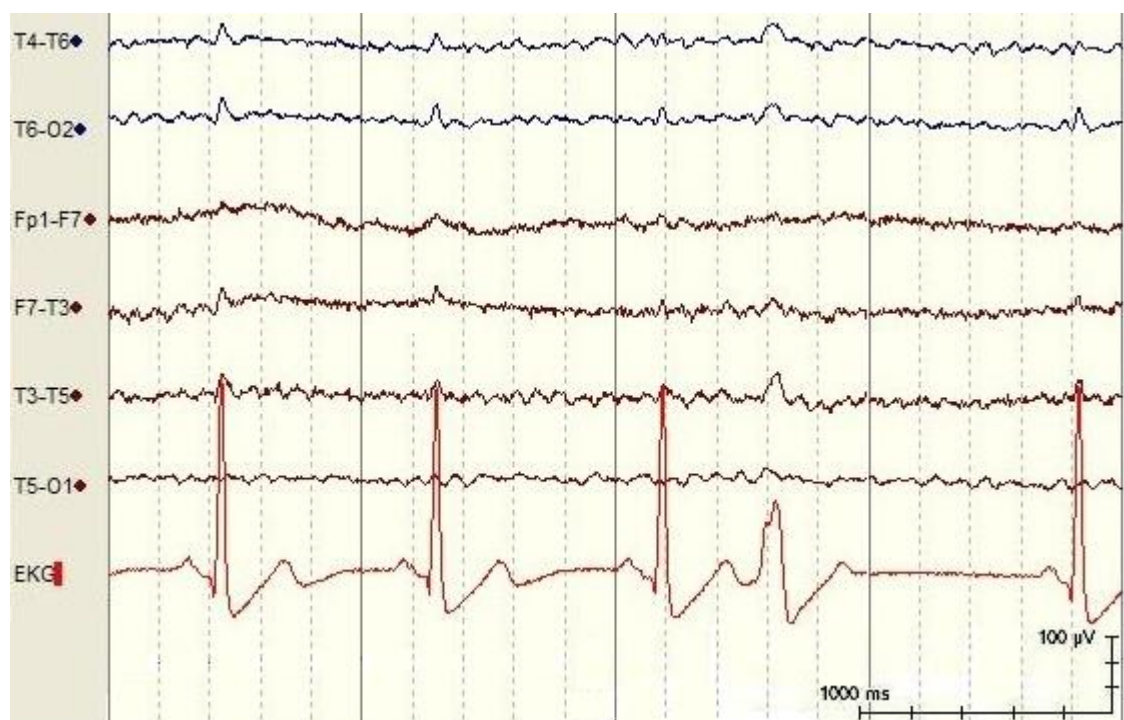
Figure 2.12. Example data including easily seen ECG artefact in many of the EEG channels used in the EEG measurement. Fourth ECG signal is an extra systole. Lowest signal in the figure is the ECG signal.
