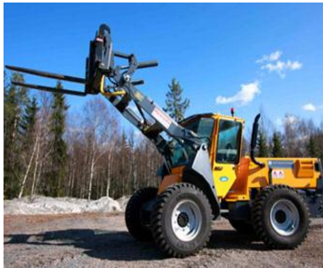
Figure 2: The wheel loader used in the GIM project (IHA machine)
