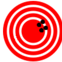
Figure 3.3 Representation of high accuracy and high precision.
