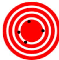
Figure 3.1 Representation of high accuracy and low precision.
