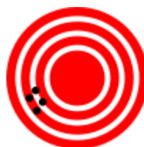
Figure 3.2 Representation of high precision and low accuracy
