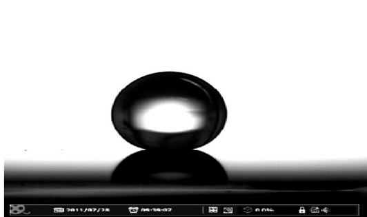
Figure 30. Water droplet on the superhydrophobic surface containing silver particles.
