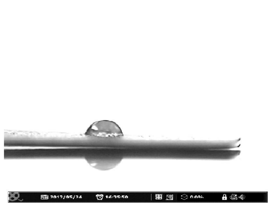
Figure 35. Water droplet on a hybrid surface that has been wiped with ethanol.
