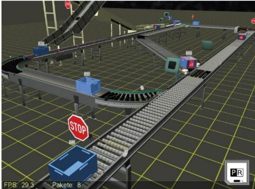
Figure 2.16. 3D monitoring system of material flow. [Feldhorst et al., 2002]
