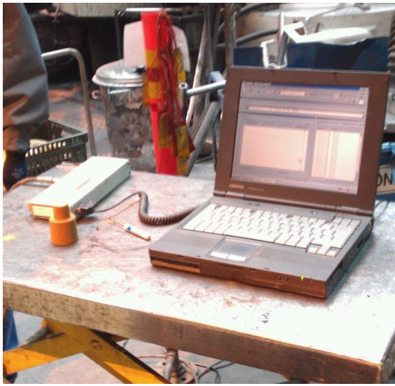
Figure 16 - The measurement setup for the thermal analysis of the casting alloys.
