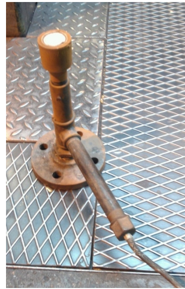
Figure 17 - The instrumentation for the thermal analysis of the casting alloys.
