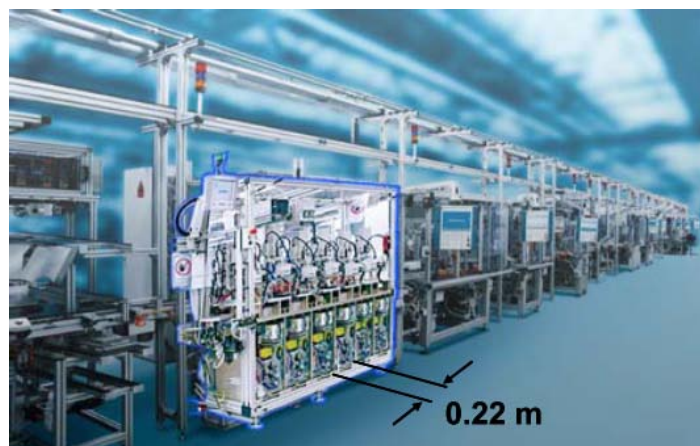
Figure 8.3. Reducing the length of an assembly line (Klemd, 2007)
